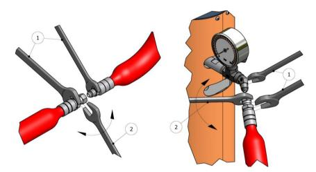
Figure 3. Hose coupling method
