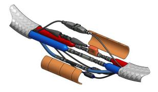
k) As soon as the connections were completed, place the protections for the union fixing them with three plastic bridles. Later cover the union with the ends of the cases.
