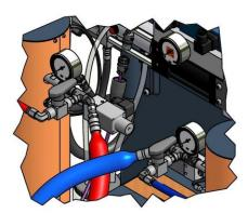
NB: To protect the TCS sensor, you must pay special attention not to kink or excessively bend the hoses. Do not roll up the hoses with a radius of under one meter / 4 feet.
