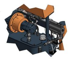
PRECAUTION! Do not fill the tank to maximum capacity (78 Lts – 20.6 gal); make sure the amount of oil is not more than 80% of its maximum capacity (63 Lts. – 16.6 gal). Use the visual level indicator of temperature on the tank as a reference, because the maximum temperature limit (80°C – 176°F) coincides with the advised capacity.
