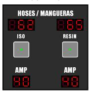
To select the temperature when the unit is working in automatic control mode, press the MODE key until the temperature flashes, select the required temperature by pressing the UP/DOWN keys and press the MODE key once more to enter the selected value into memory. Repeat the process to select the Amps. When the unit is in automatic mode, the value of the power must be set between 45 and 50 Amps.
