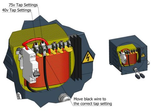
installed. Before starting up the unit, make sure that the connection made in the factory adapts to the total length of hose installed. If you add or eliminate sections of hose, make sure the output voltage of the transformer to which it is connected is suitable for the resulting total length. Otherwise, change the connection.
