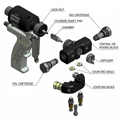
**PRECAUTION:** To avoid spilling the rest of the product which has accumulated in the side cartridges onto the floor, always remove the coupling block and the side cartridges on a waste vessel.
