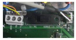
NOTE: The unit must be turned off to be able to work on the DIP selector.
