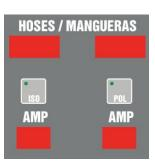
The push-buttons turn on or off the hose heating system of each
