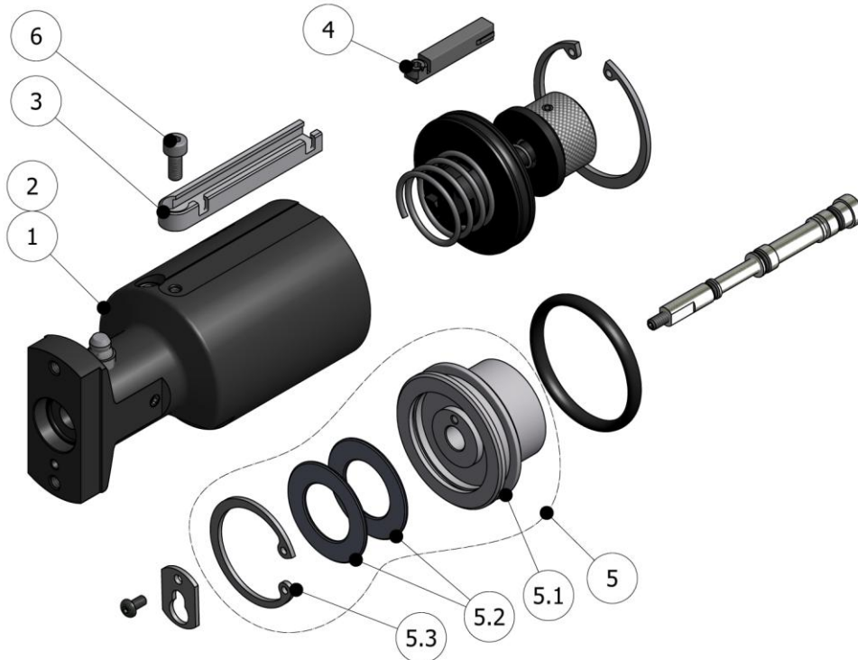
Figure 5. (OPTIONAL) Magnetic Switch Assembly, Exploded View
